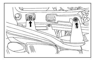
3. Remove the two screws retaining the headlamp assembly.
